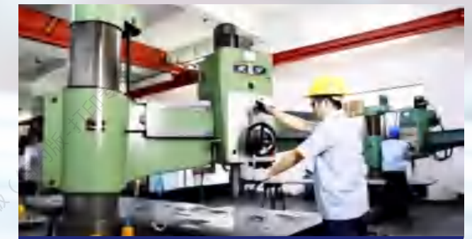
铣钻床-摇臂钻床（共4台） Milling and drilling machine - Rocker arm drilling machine (4 units in total)
