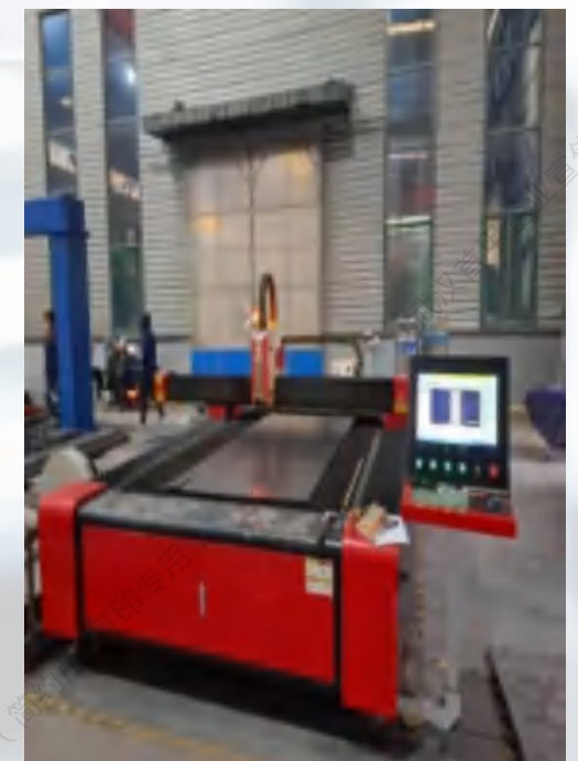
OFFP-B敞开式光纤激光切割机一台 One OFFP-B open type fiber laser cutting machine
