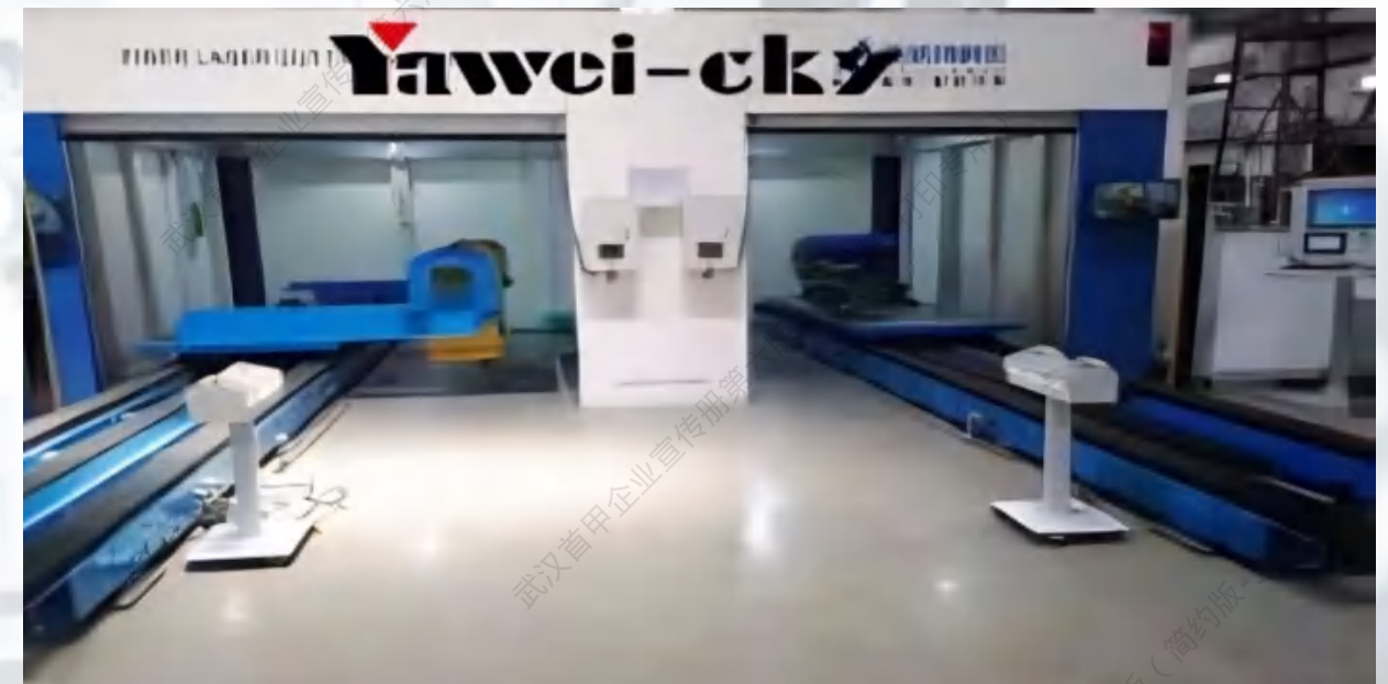
HLTD-153三维五轴全自动激光切割机一台 One HLTD-153 three-dimensional five axis fully automatic laser cutting machine
